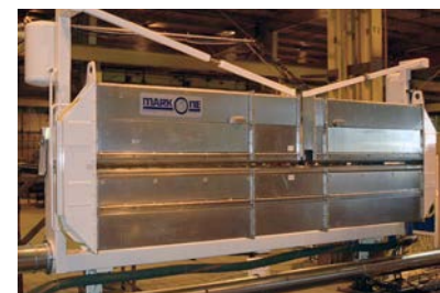
Programmable Spray Lubricator (Re-Oiler)
